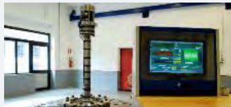
Full scale fatigue test of axles
